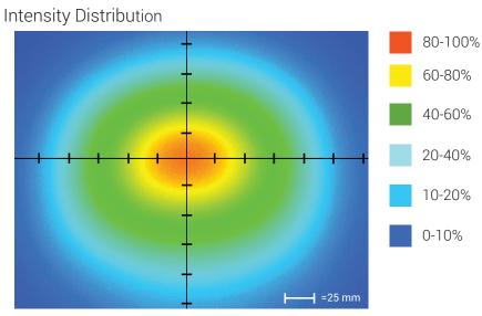
Optical measurement taken using SL-S100150M-WHI @ 300 mm
