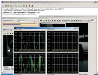
Multiple Channel Data Acquisition Synchronized To Each Frame
