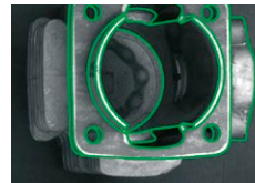
Localization of a known object with 3D matching.
