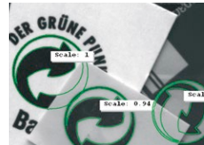
HALCON's perspective deformable matching robustly localizes objects with perspective distortions.
