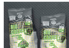
HALCON's local deformable matching finds objects with surface deformations.
