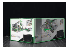
HALCON's descriptor-based matching locates planar objects extremely fast.
